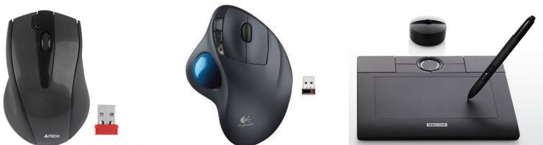
Figure 3.6 On the left is an example of a wireless optical mouse, trackball is in the middle and tablet on the right
