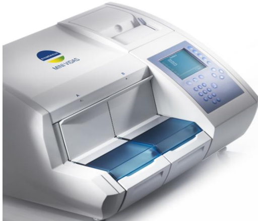
Figure 5: The automated VIDAS® instrument. All of the assay steps are performed automatically by the instrument after inserting the SPR®s and strips . (Photos: bioMérieux, France; author)
