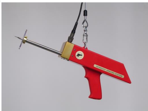
HENNESSY GRADING PROBE
